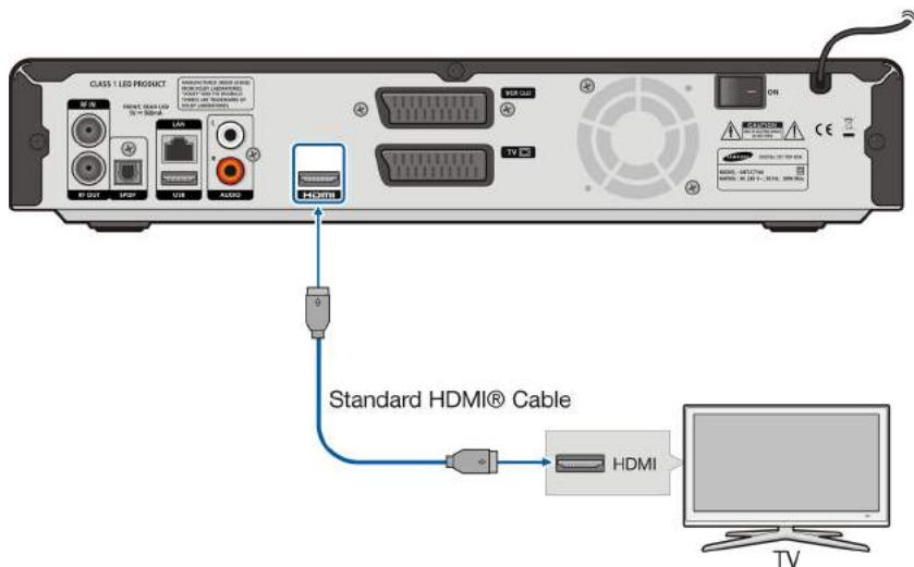
Connect the **HDMI** port on the rear of the STB to the **HDMI** port of the TV by using a standard HDMI® cable.
