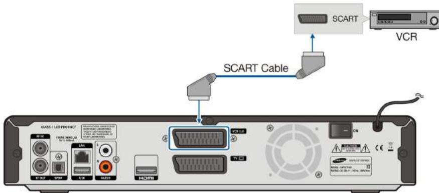
Connect the **VCR SCART** port of the STB to the **SCART** port of the VCR by using a SCART cable.
