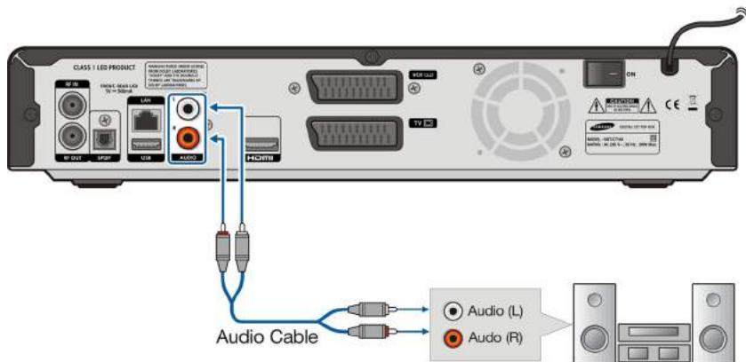
Using the audio cable, connect the **AUDIO** port at the rear of the STB to the **Audio** port of an audio.
