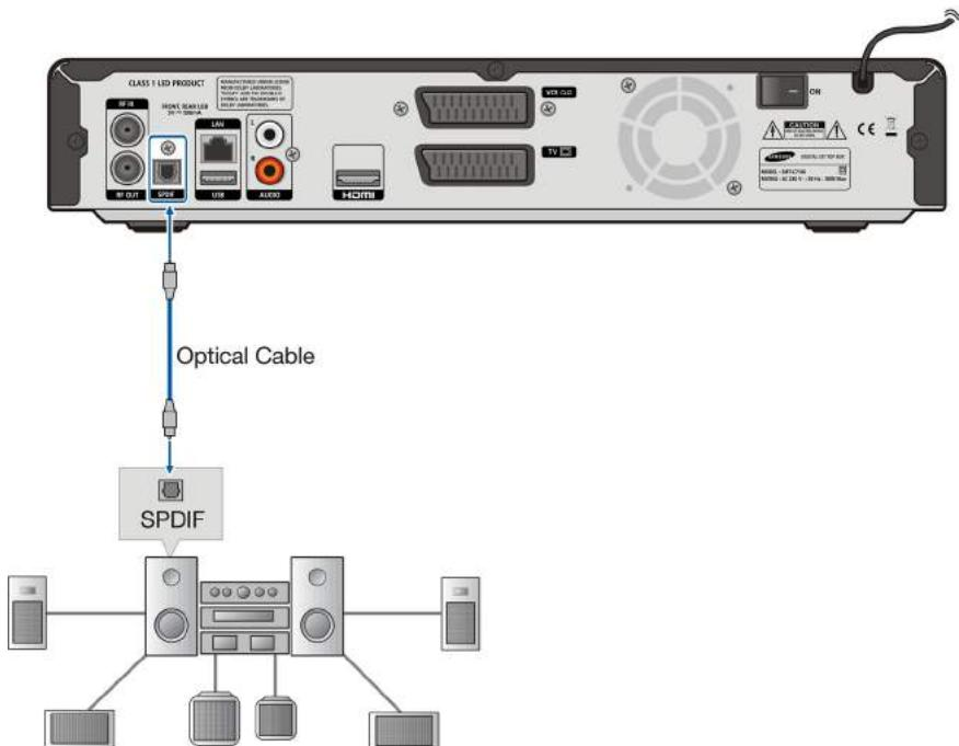
Using the optical cable for digital audio, connect the **DIGITAL AUDIO OUT** port at the rear of the body to the **Digital audio in (SPDIF)** port of a Dolby Digital audio.
