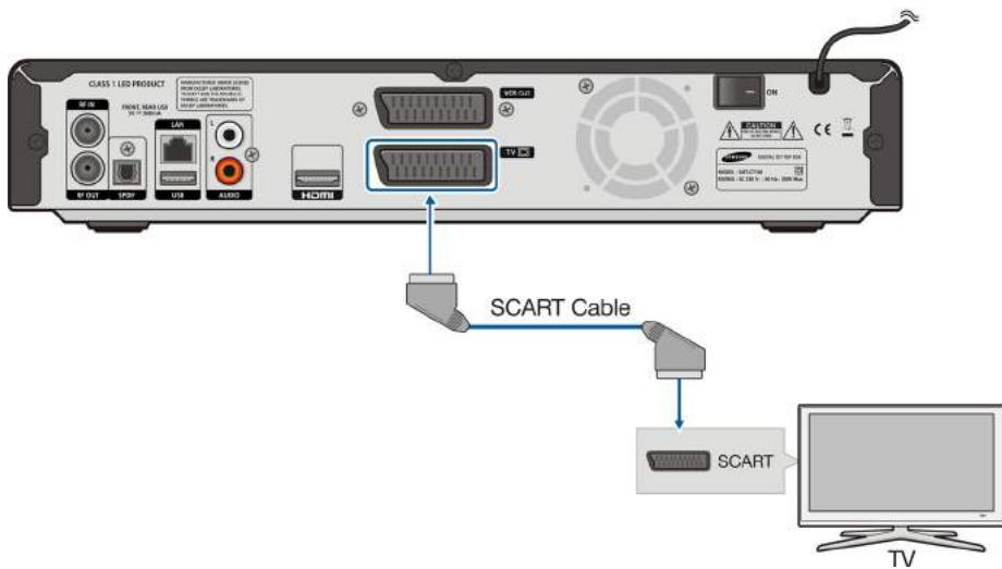
Connect the **TV SCART** port on the rear of the STB to the **SCART** port of the TV by using a SCART cable.
